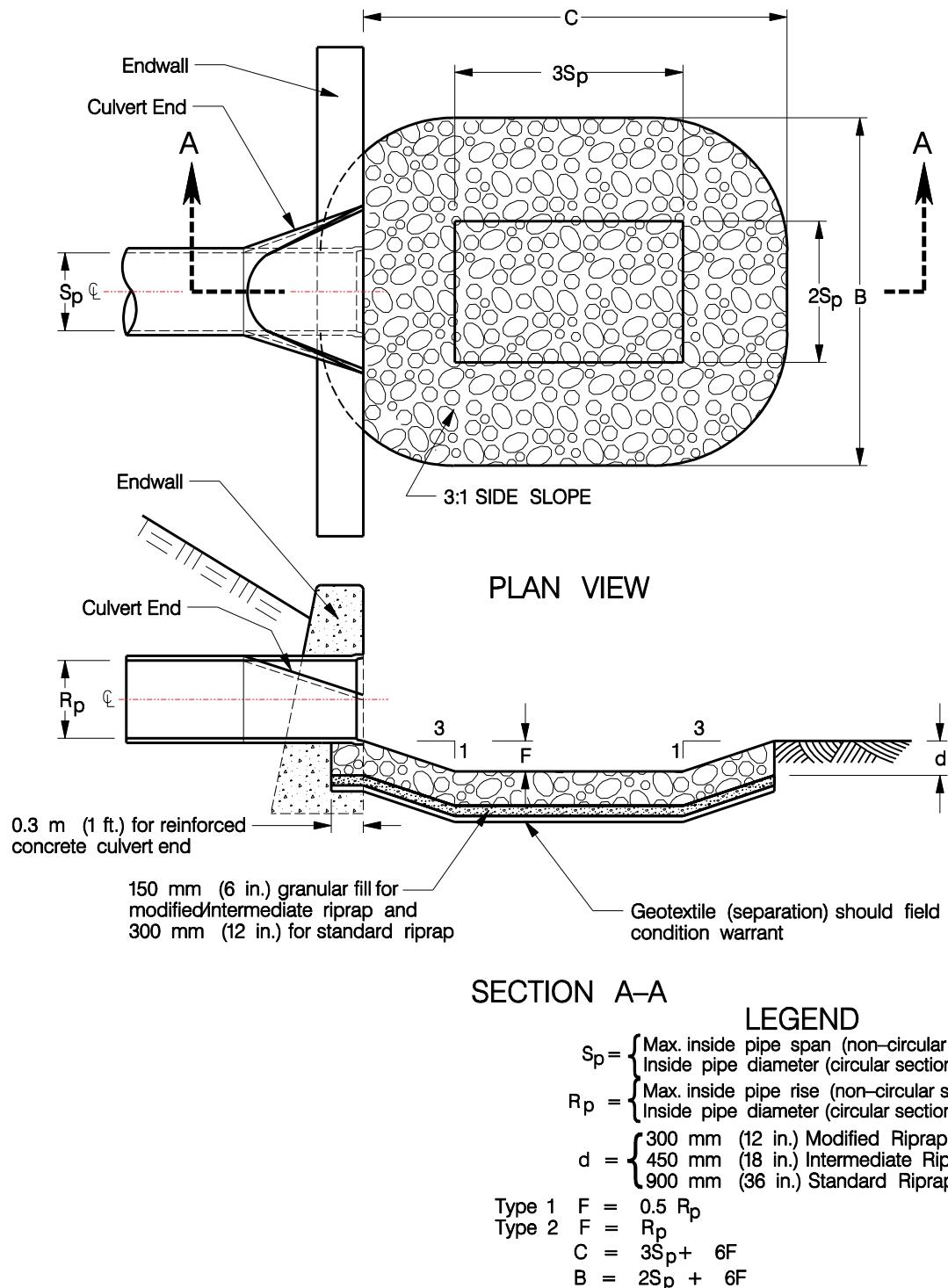
Figure 11-15 Preformed Scour Hole Type 1 and Type 2
