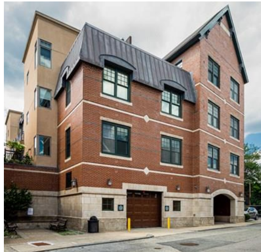
Figure 80. The garage door on this building in Winchester, MA was designed as an integral part of the façade. The garage entrance and the lobby entrance (arched passage on the right) are of similar size and their lintels have a similar design. The central placement of the garage entrance is highlighted by the diamond details above it, while the square windows on either side of it align with the outside edges of the windows above. (Google Streetview)
