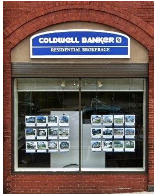
Figure 46. A central mullion can divide a horizontally oriented window into vertical panels (Google Streetview)
