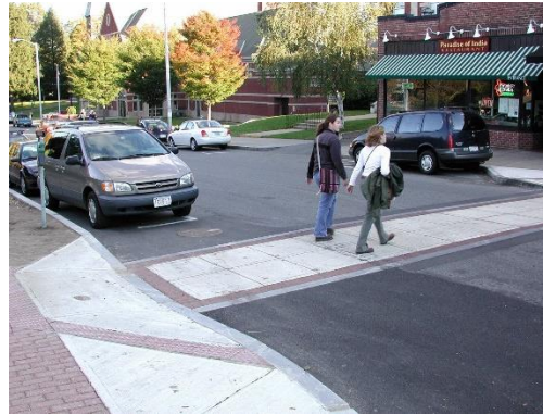
Figure 73. A crosswalk in Amherst, MA is built out of concrete with brick edging making it highly visible and more durable than a painted crosswalk.
