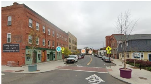
Figure 70. Example of curb extensions and a raised crosswalk in Northampton MA. The crosswalk is surfaced with colored and textured pavement. Impact on snow removal is often a concern when these elements are proposed. In Northampton, City snowplows are able to negotiate the curb extension and raised crosswalk without issues.
